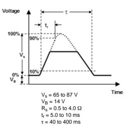
Figure 17. ISO 7637–2, Pulse 5b Waveform
