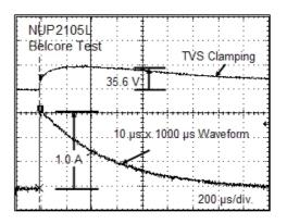
Figure 19. Test Response of the NUP2105L to the 10 x 1000 µs Waveform
