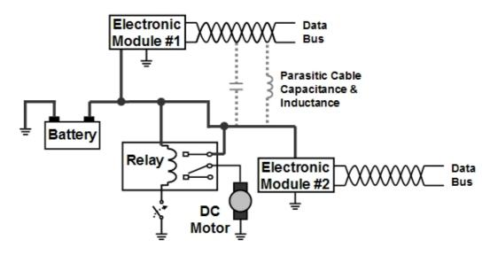
Figure 2. External system noise can easily enter an electronic module from conduction and coupling via the power supply and data cables.
