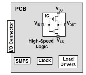
Figure 3. Common PCB Noise Sources
