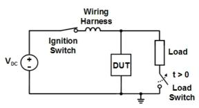
Figure 7. Test pulse 2a of ISO 7637–2 represents the surge produced by the inductance of the wiring when power is removed from a load that is connected in parallel with an electronic module.
