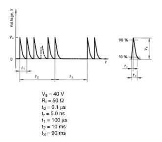
Figure 14. ISO 7637-3, Pulse 3b Waveform
