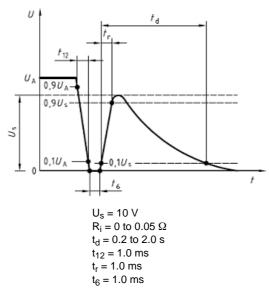
Figure 10. ISO 7637-2, Pulse 2b Waveform
