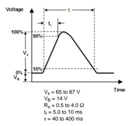
Figure 16. ISO 7637-2, Pulse 5a Waveform
