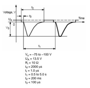
Figure 6. ISO 7637-2, Pulse 1 Waveform
