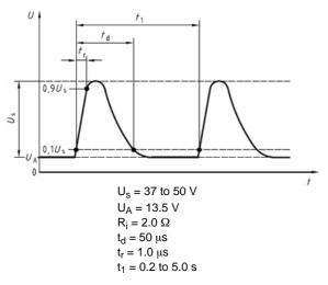
Figure 9. ISO 7637-2, Pulse 2a Waveform
