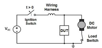
Figure 8. Test pulse 2b of ISO 7637–2 represents the surge produced by the inductance of the wiring when power is removed from both the parallel load and the electronic module.
