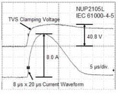
Figure 20. Test Response of the NUP2105L to the 8 x 20 µs Waveform
