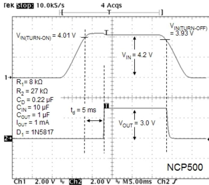
Figure 7. The circuit in Figure 3 turns on only after a sufficient input voltage is reached and shuts down immediately after the input becomes insufficient.
