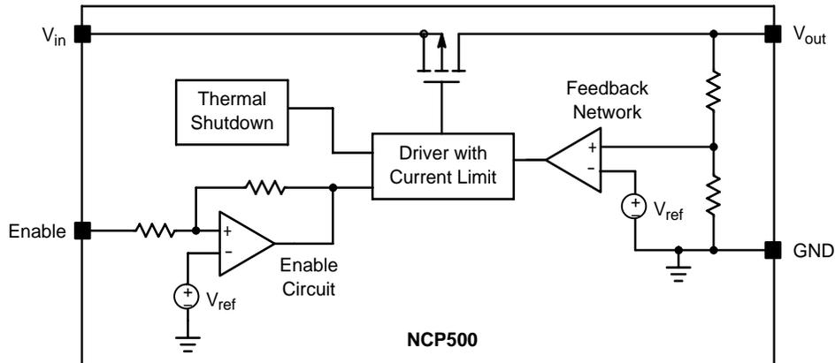
**Figure 4. Block Diagram of the NCP500 Voltage Regulator**
