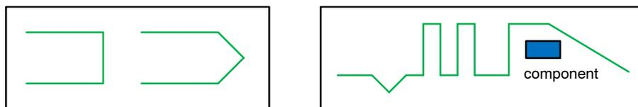
**Figure 4. Improper Ways of Trace Routing**
