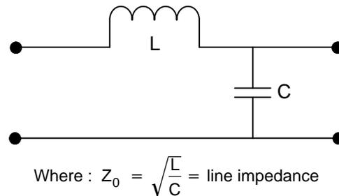
Figure 1. Lossless Transmission Line – Equivalent Circuit
