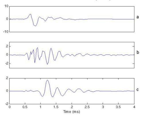
Figure 3. Impulse responses from three different hearing aid styles: a) ITC, b) ITE, and c) BTE.
