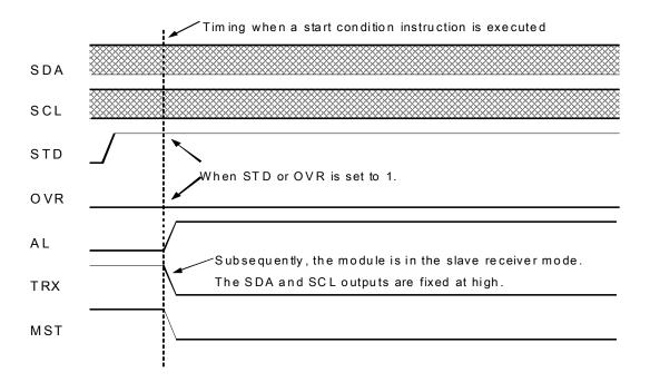
Figure 3.22.9 Arbitration Lost During Start Condition Generation <1>
