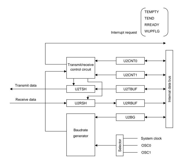
Figure 3.19.1 UART2 Block Diagram
