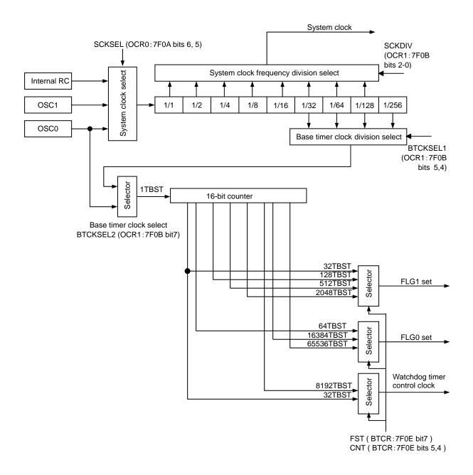
Figure 3.17.1 Base Timer Block Diagram
