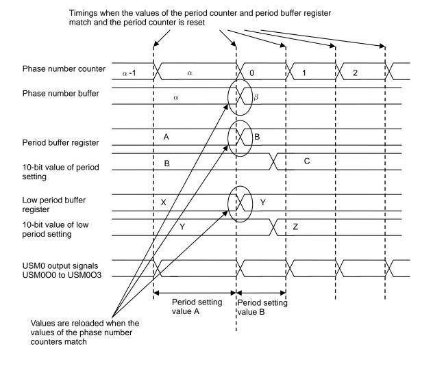
Figure 3.26.4 Stepping Motor Mode Reload Timing
