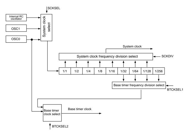
Figure 4.2.1 System Clock Generator Block Diagram
