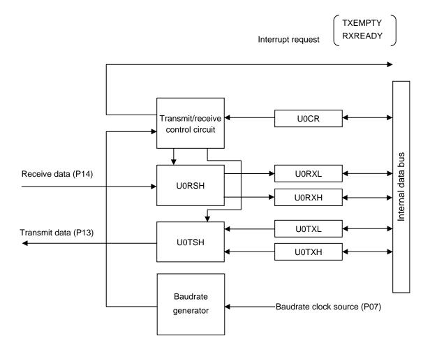
Figure 3.18.1 UART0 Block Diagram
