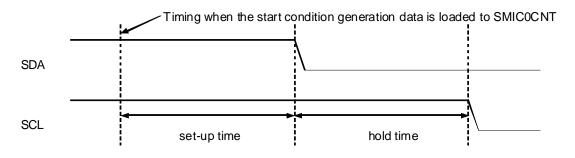
Figure 3.22.5 Start Condition Generation Timing Diagram
