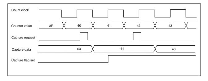
Figure 3.14.1 Capture Timing
