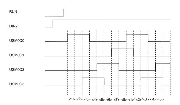
Figure 3.26.11 Mode 1 Operation Start Time Waveforms (Reverse Rotation)
