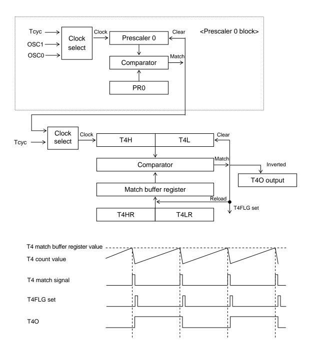
Figure 3.16.1 Timer 4 Block Diagram
