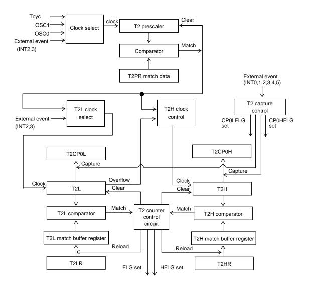
Figure 3.14.2 Timer 2 Block Diagram
