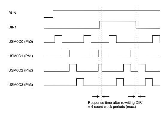
Figure 3.26.7 Reverse Rotation as Controlled by DIR1
