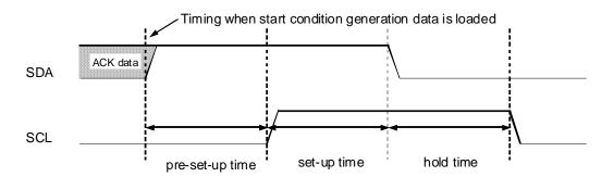
Figure 3.22.6 Restart Condition Generation Timing
