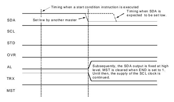
Figure 3.22.10 Arbitration Lost During Start Condition Generation <2>
