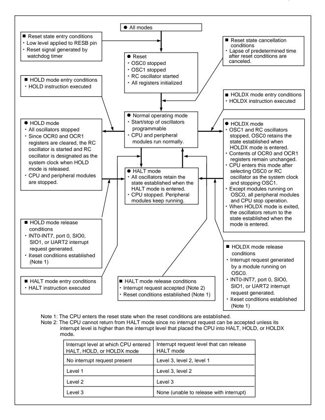
Figure 4.3.1 Standby Mode State Transition Diagram
