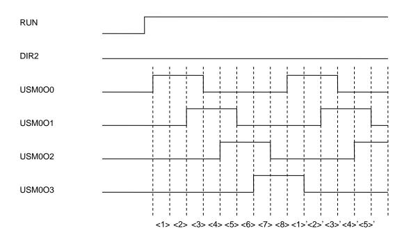
Figure 3.26.10 Mode 1 Operation Start Time Waveforms (Forward Rotation)
