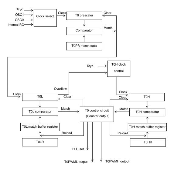
Figure 3.12.1 Timer 0 Block Diagram
