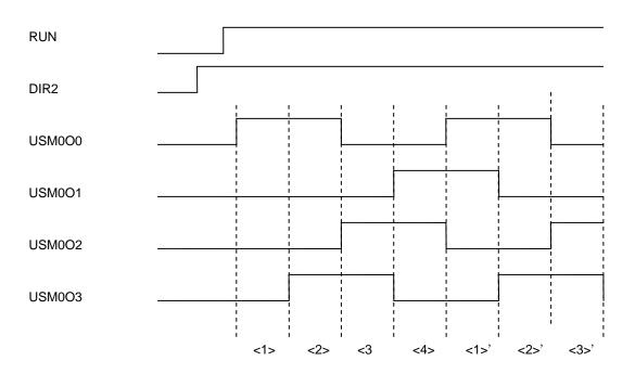
Figure 3.26.13 Mode 2 Operation Start Time Waveforms (Reverse Rotation)
