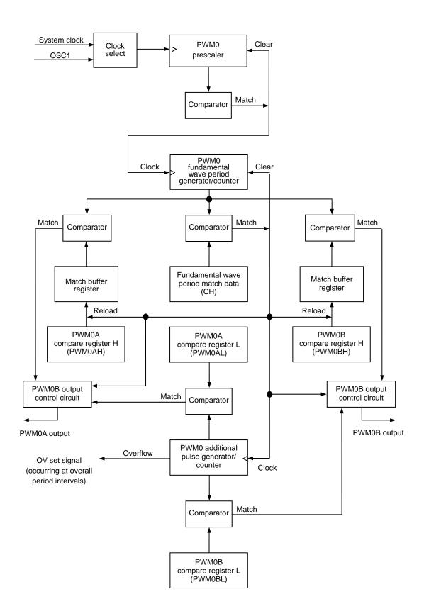
Figure 3.23.1 PWM0 Block Diagram
