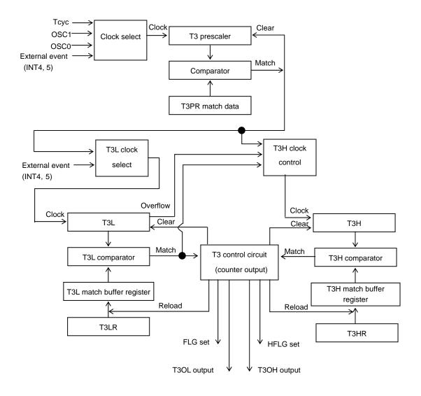
Figure 3.15.1 Timer 3 Block Diagram
