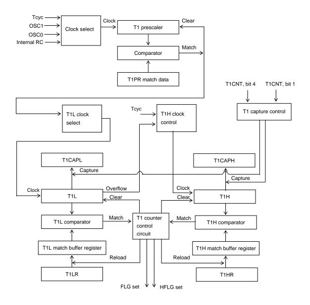
Figure 3.13.1 Timer 1 Block Diagram
