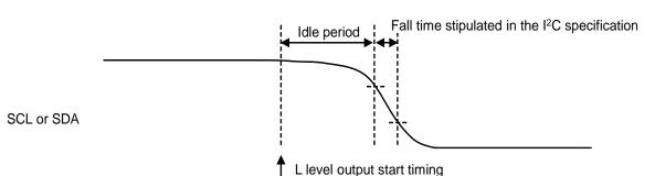
Figure 3.22.2 I<sup>2</sup>C Port Falling Waveform
