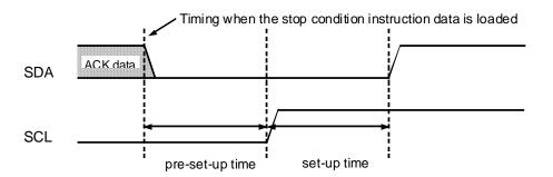
Figure 3.22.7 Stop Condition Generation Timing
