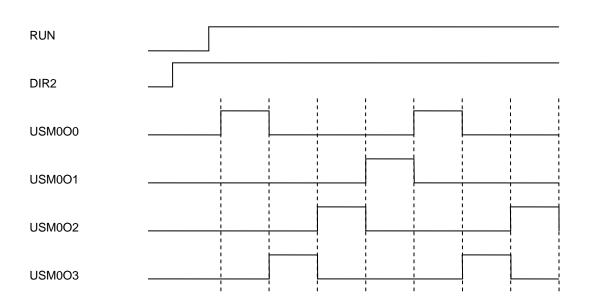
Figure 3.26.9 Mode 0 Operation Start Time Waveforms (Reverse Rotation)
