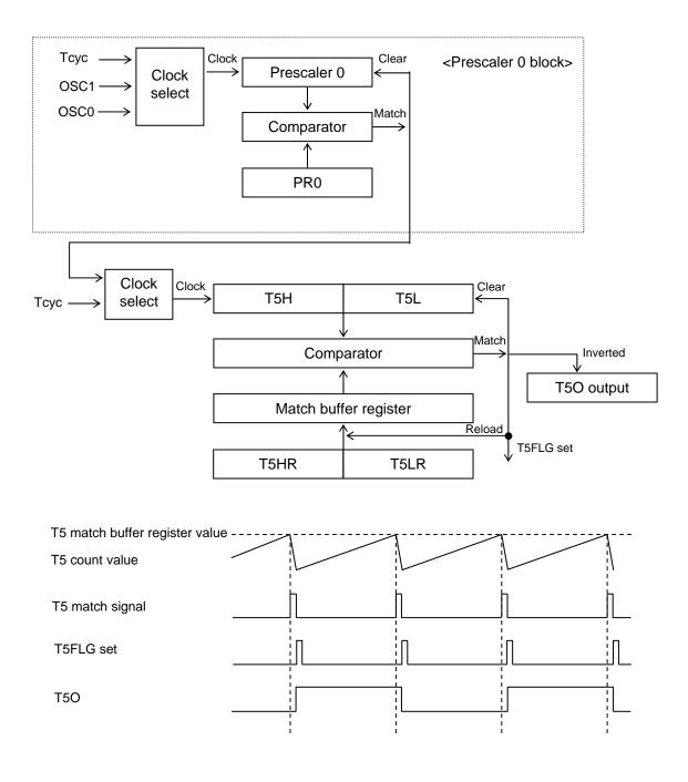
Figure 3.16.2 Timer 5 Block Diagram
