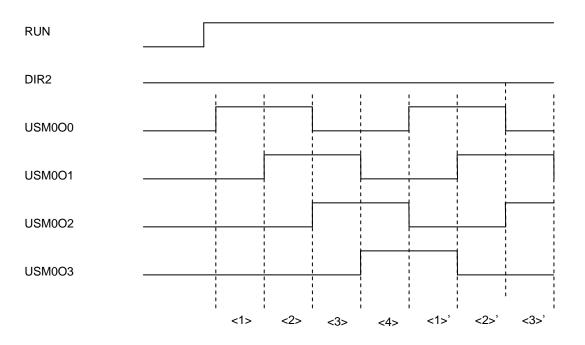
Figure 3.26.12 Mode 2 Operation Start Time Waveforms (Forward Rotation)
