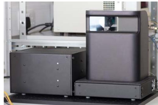
Figure 1. The ON Semiconductor Gen3 LiDAR Demonstrator
