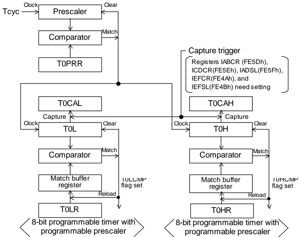
Figure 3.3.1 Mode 0 Block Diagram (T0LONG = 0, T0LEXT = 0)
