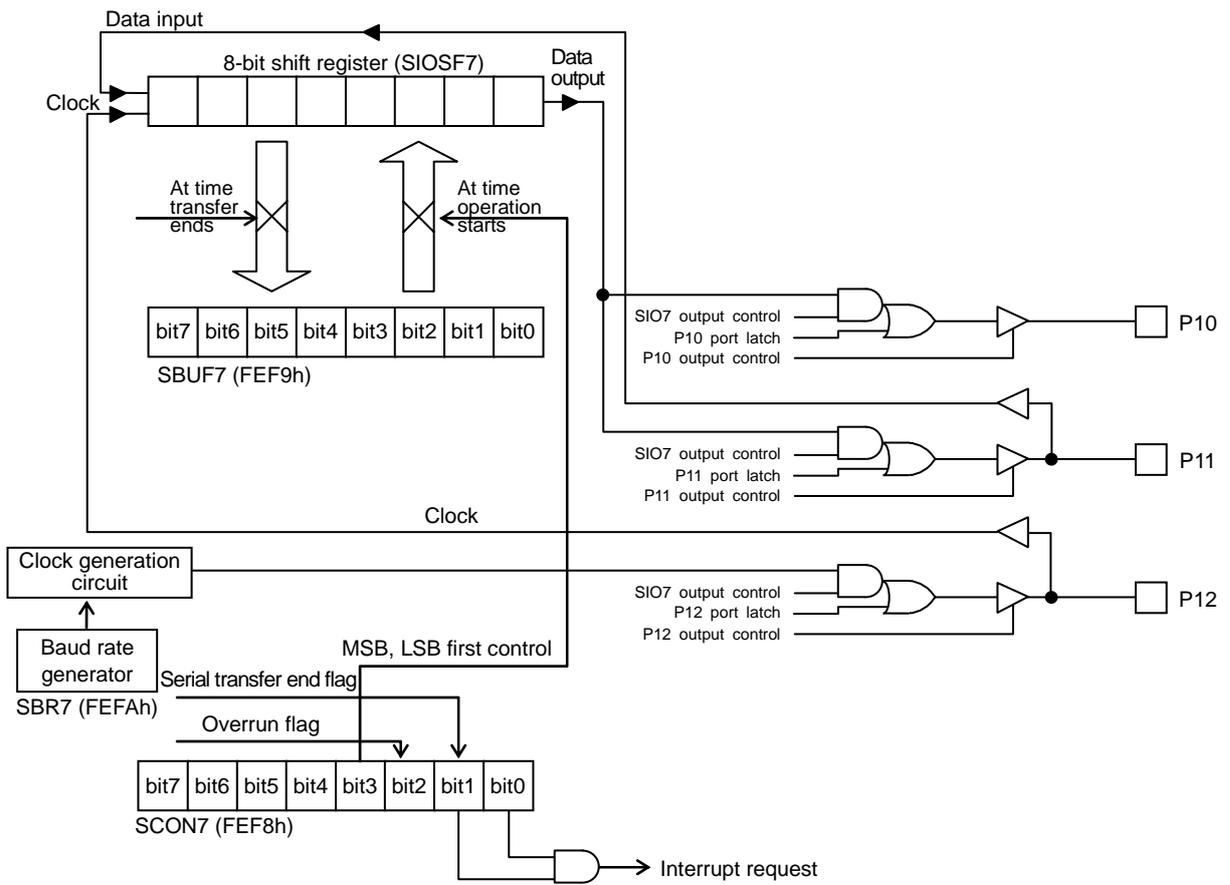
**Figure 3.5.1 SIO7 Synchronous 8-bit Serial I/O Block Diagram**
