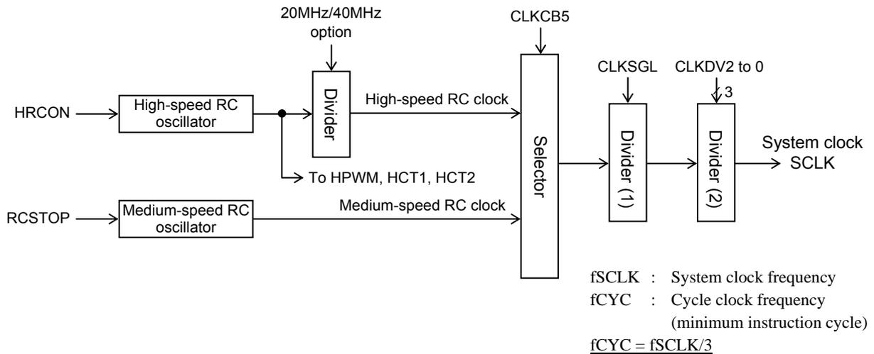
Figure 4.2.1 System Clock Generator Block Diagram
