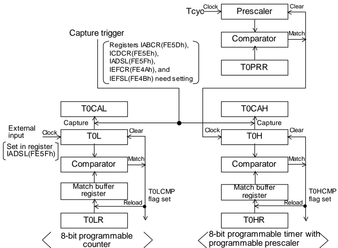
Figure 3.3.2 Mode 1 Block Diagram (T0LONG = 0, T0LEXT = 1)
