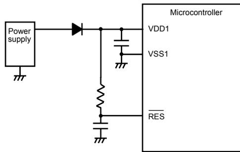
Figure 4.5.4 Example of Power Interruption / Voltage Fluctuation Countermeasures
