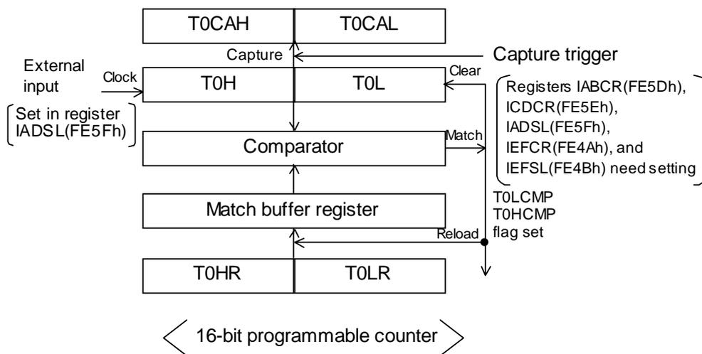
Figure 3.3.4 Mode 3 Block Diagram (T0LONG = 1, T0LEXT = 1)
