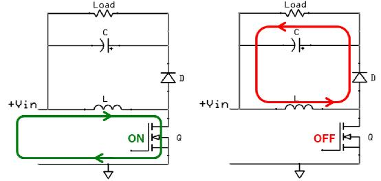
This Design Note describes such a circuit which operates from 10 to 25 V input and produces 15 to 22 V in order to drive a string of several power LEDs at up to 3 A.
