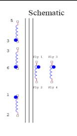
Bobbin Pinout - Bottom View
