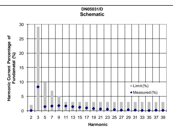
Figure 2: EN61000-3-2 Class C Input Current Harmonic Test (Vin=230 Vac, 50 Hz, Iout =704 mA @36.1V)
