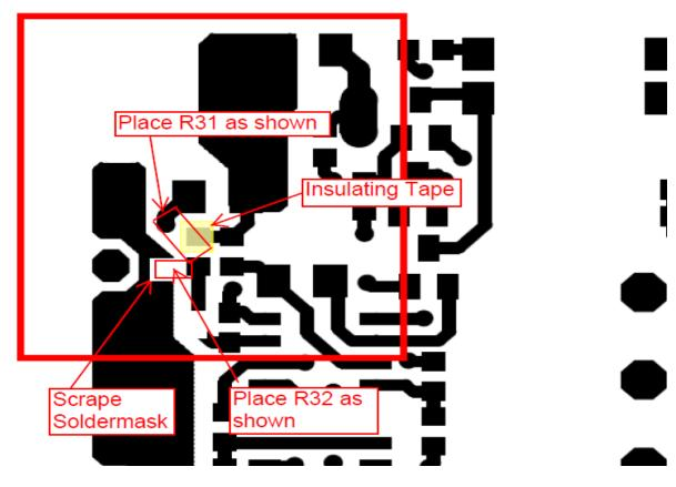
Figure 4. Detail of Rework Area in Figure 3
