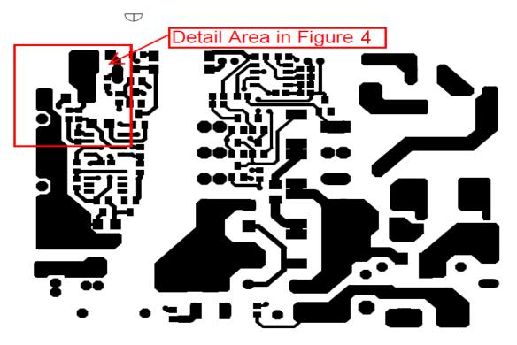
Figure 3. Demo Board Bottom Side Copper
