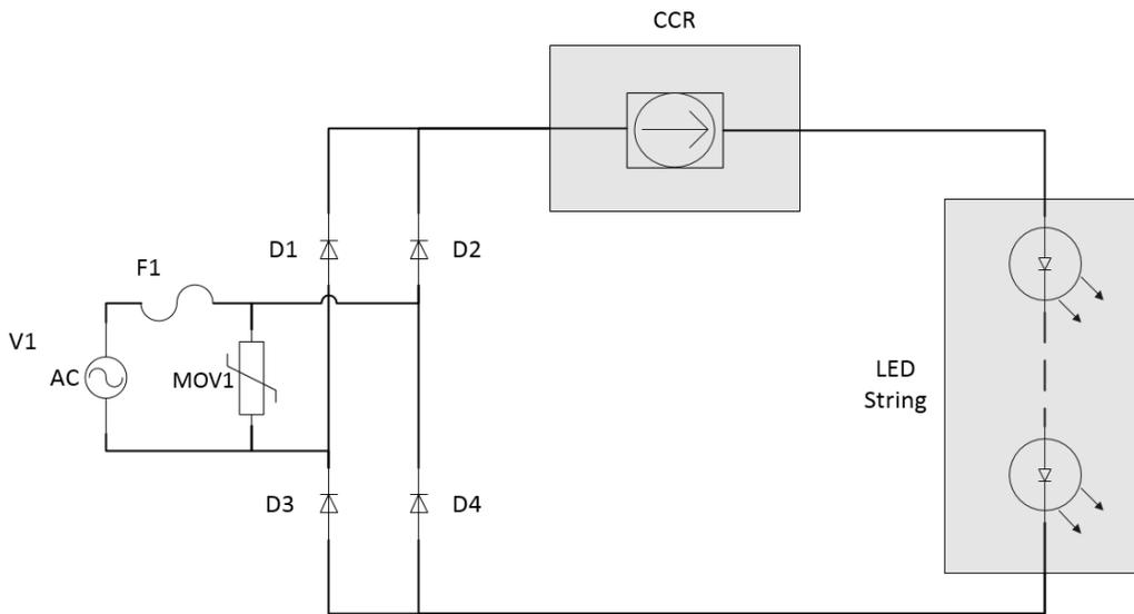
Figure 1 – General “Straight Circuit” CCR-based LED Driver Schematic
