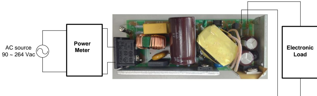
Figure 2. Test setup
