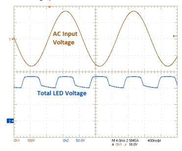
The circuit is operating with an AC Input Voltage of 120 Vac (rms). Total LED voltage is approximately 136 V.
