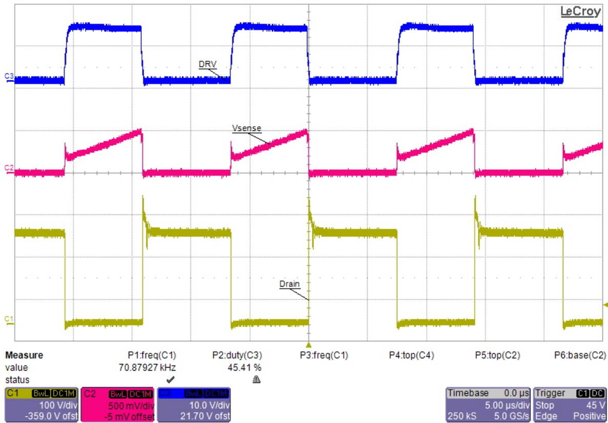
Figure 7. CCM Operation at Full Load (3.5 A) and 85 V/50 Hz Input
