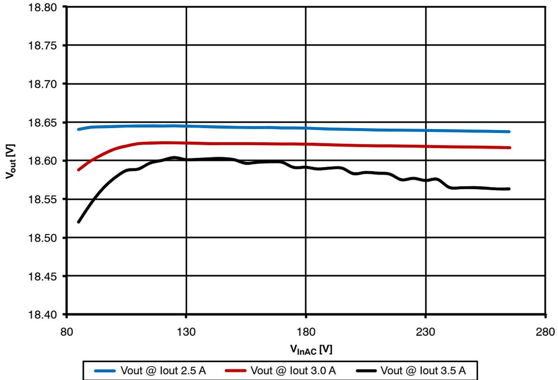
Figure 4. Line Regulation for High Output Loads
