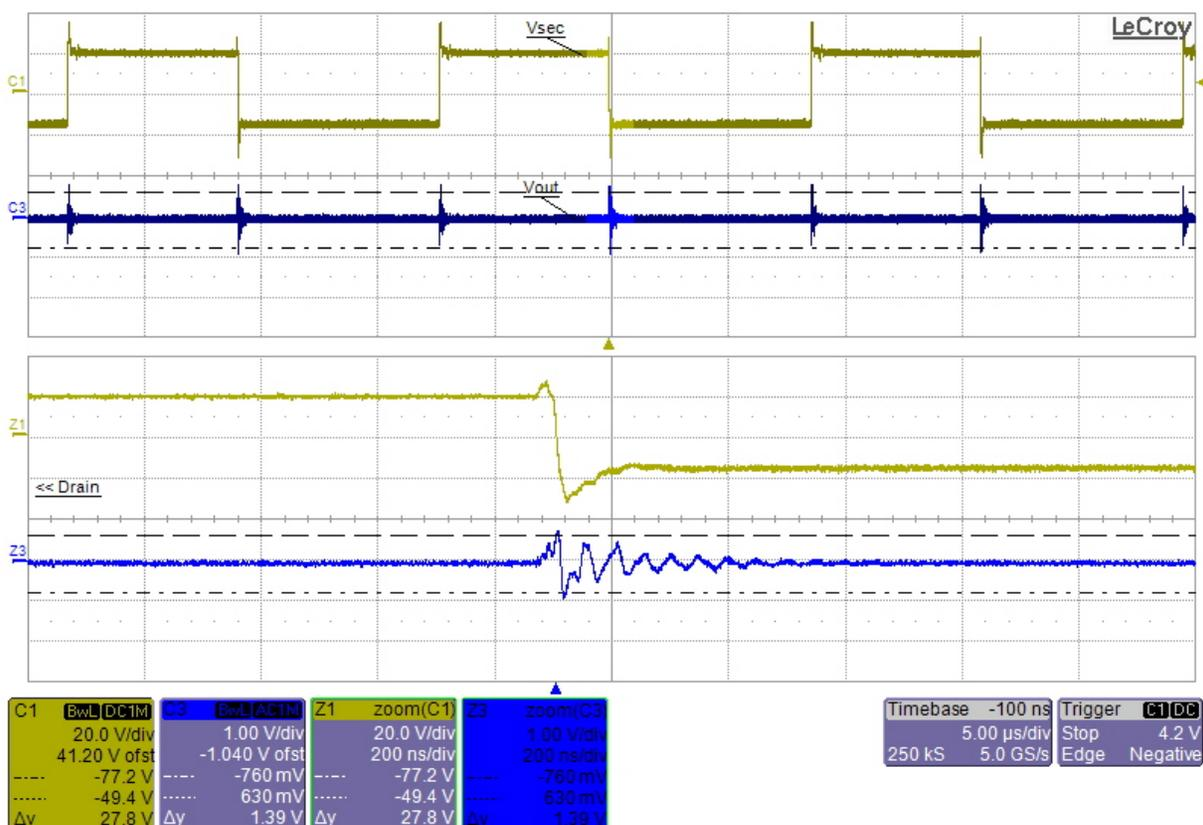
**Figure 25. Detail of the Output Voltage Ripple and Voltage Across Secondary Winding of Transformer at 85 V/50 Hz Input with 3.5 A Output Current Loading (the ringing is caused by the secondary diode reverse recovery)**
