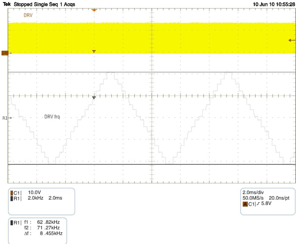
Figure 24. Frequency Deviation of the Frequency Jittering
