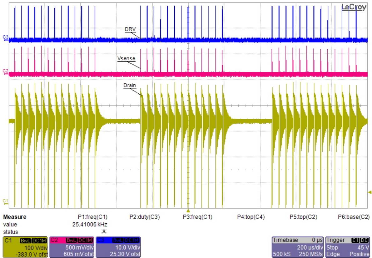
Figure 17. The Skip Mode Starts at 0.25 A of Load Current at 230 V/50 Hz Input
