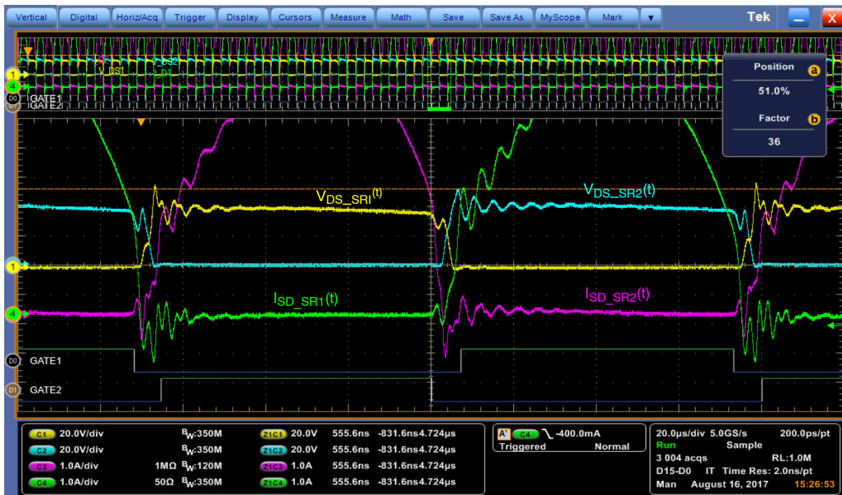
Figure 29. Synchronous rectifier operating waveforms, I_{OUT} = 8\text{ A} , V_{IN} = 120\text{ V} ,
