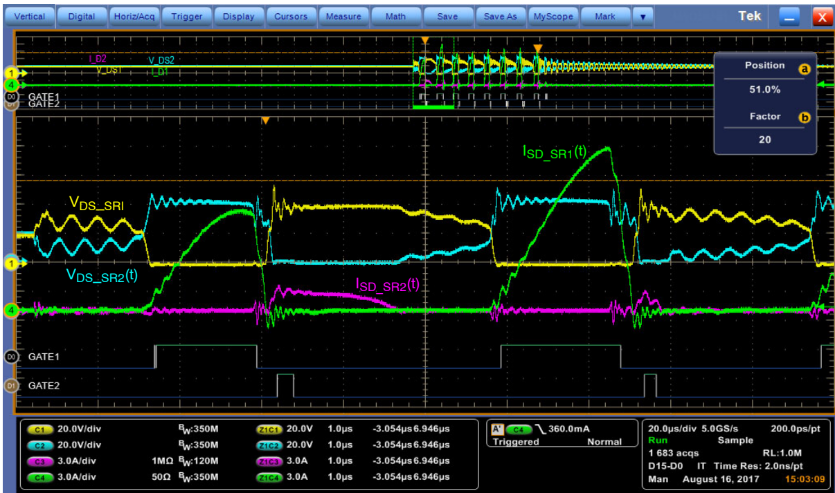
Figure 28. Synchronous Rectifier Operating Waveforms – SKIP MODE I_{OUT} = 100 \text{ mA} , V_{IN} = 120 \text{ V} ,
