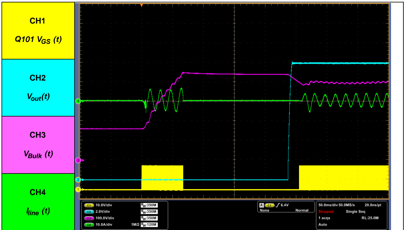
Figure 37. 110 V AC/ Load 20 A, PFC/ LLC START-UP (No inrush limiter)
