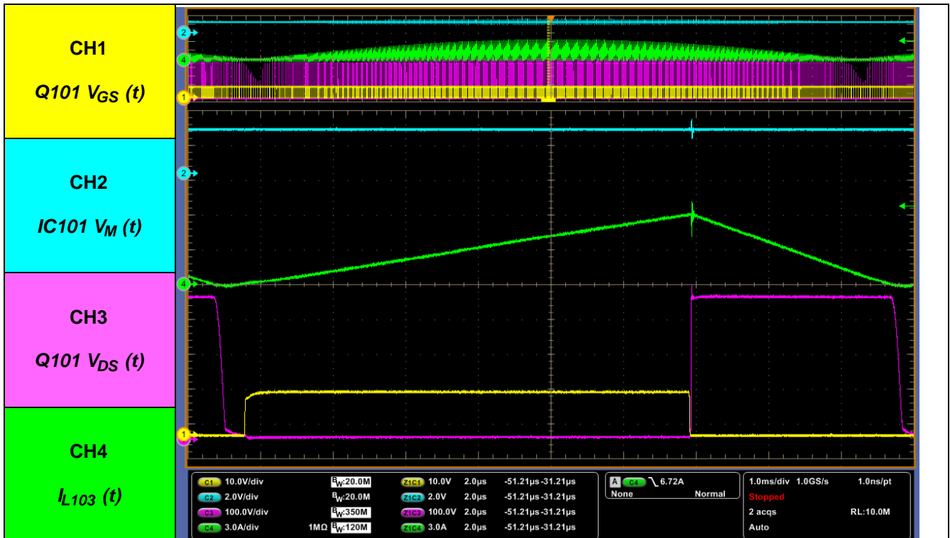
Figure 39. 90 V AC/ Load 13 A, PFC CrM MODE – before entering CCM
