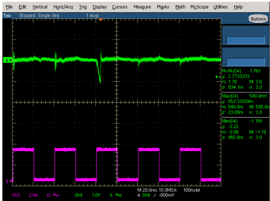
Figure 38. 37 Vin 9 Vout Transient Response
