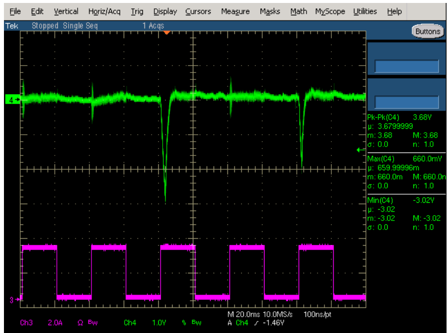
Figure 45. 48 Vin 15 Vout Transient Response
