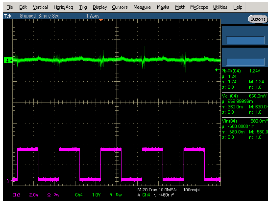
Figure 36. 48 Vin 5 Vout Transient Response
