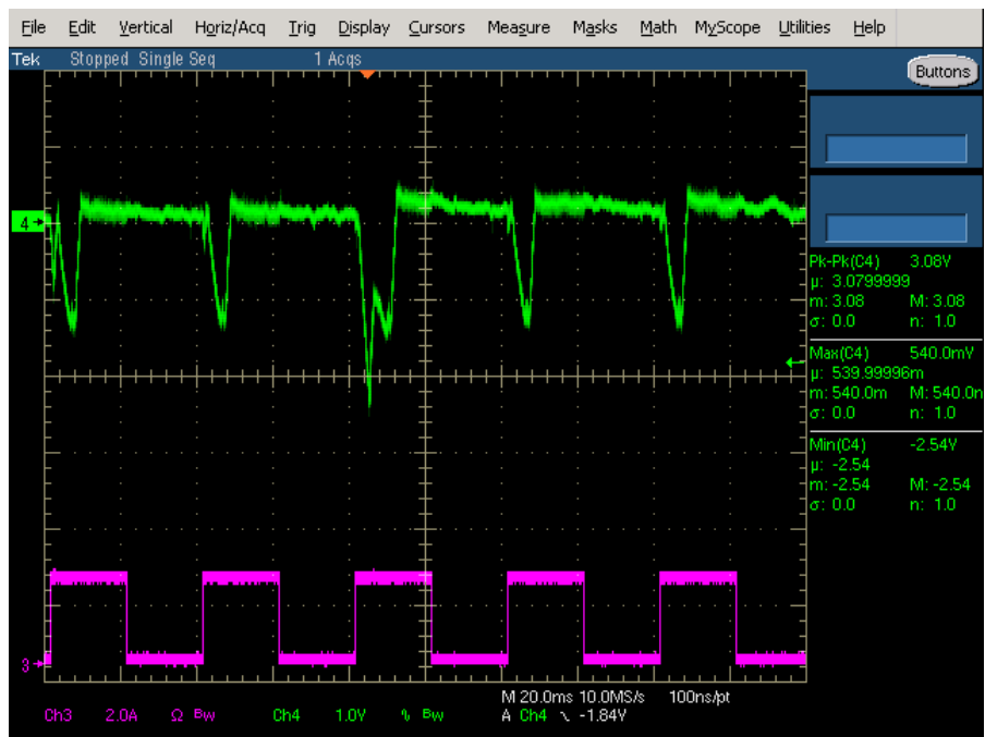
Figure 48. 48 Vin 20 Vout Transient Response
