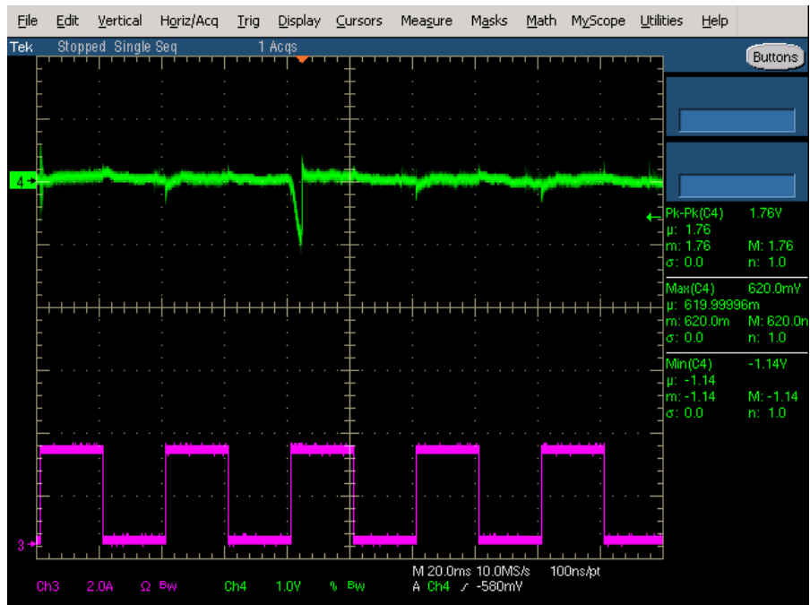
Figure 39. 48 Vin 9 Vout Transient Response
