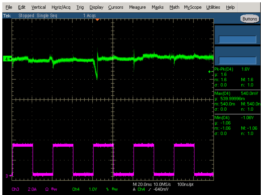
Figure 40. 57 Vin 9 Vout Transient Response
