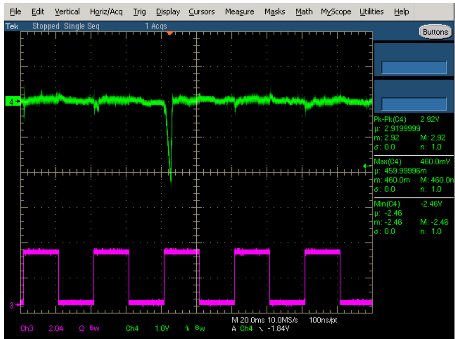
Figure 43. 57 Vin 12 Vout Transient Response
