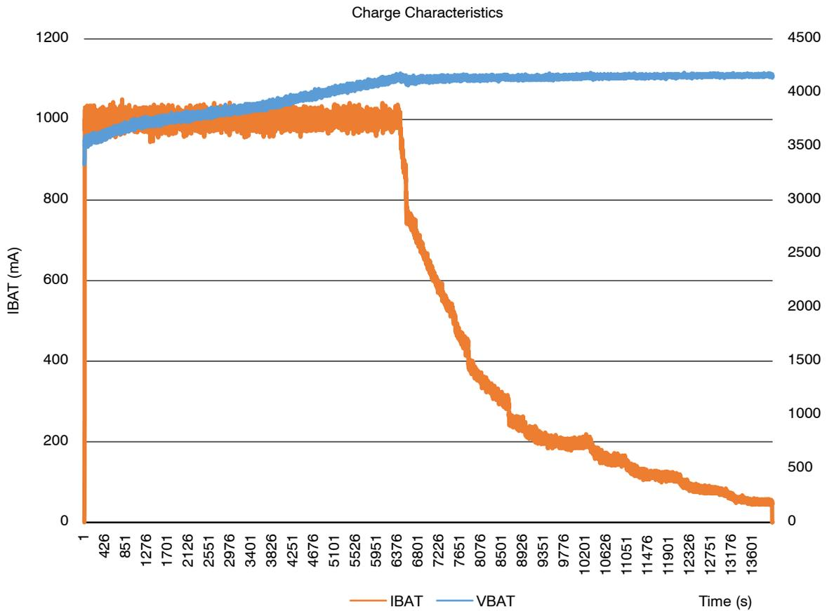
Figure 25. Charge Characteristic (Charge at 1000 mA)
