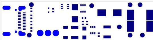
Figure 9. Solder Layer (Top Layer)
