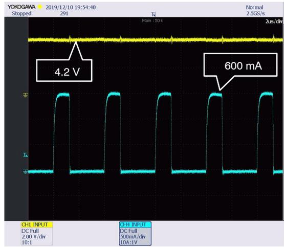
Figure 35. Waveforms for Medium Mode (LED Current ~600mA)
