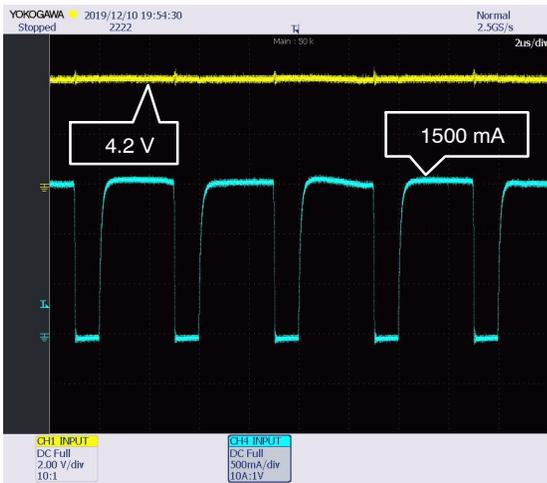
Figure 34. Waveforms for High Mode (LED Current ~ 1500 mA)
