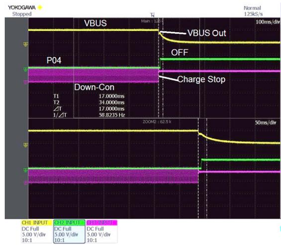
Figure 28. Disconnecting VBUS During Buck Charge Changes the Device to Standby Mode
