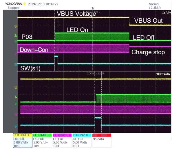
Figure 33. Initially LED is OFF and Battery is Charging. Pass-through Starts and the LED Turns ON when the Switch is Enabled
