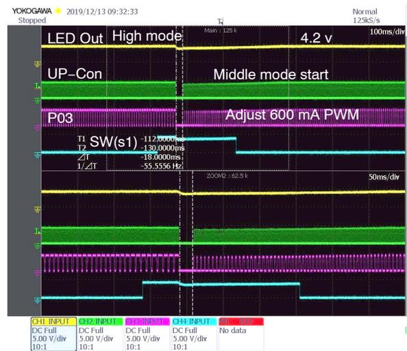
Figure 30. Switch to Middle Power Mode by Pressing Key During High Power Mode
