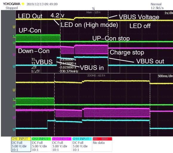
Figure 32. Pass-through Starts when VBUS is Inserted while LED is ON
