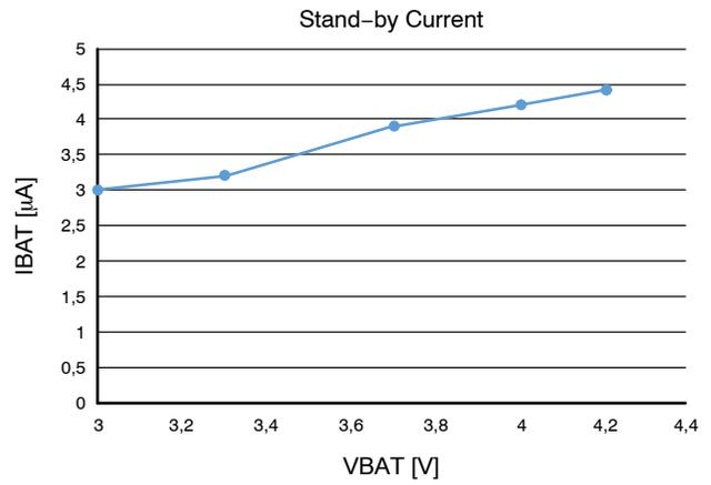
Figure 24. Stand-by Current (Lib-protection IC Included)
