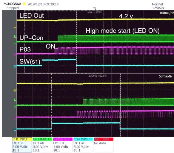
Figure 29. LED ON (High Power Mode) by Pressing Key During Standby
