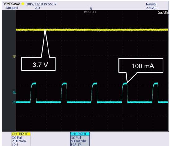
Figure 38. Waveforms for Flash2 Mode (LED Current = 100 mA)
