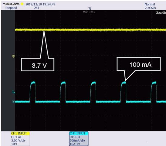
Figure 36. Waveforms for Low Mode (LED Current ~ 100 mA)
