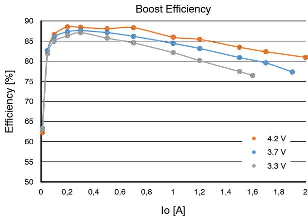
Figure 23. Boost Efficiency
