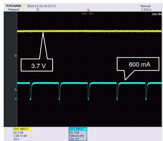
Figure 37. Waveforms for Flash1 Mode (LED Current ~ 600 mA)
