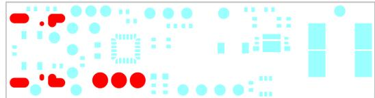
Figure 10. Solder Layer (Bottom Layer)
