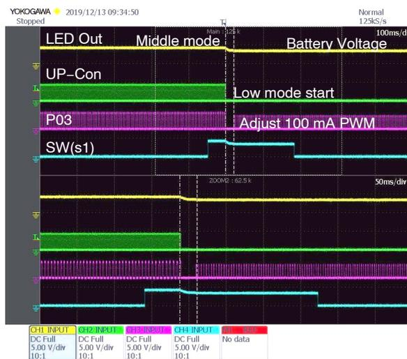
Figure 31. Press Key in Middle Power Mode to Switch to Low Power Mode (Up-con is Disabled on this Mode)
