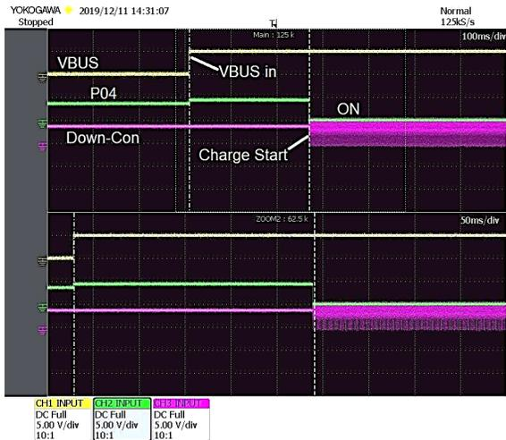
Figure 27. Connecting VBUS During Standby to Start the Buck Charge
