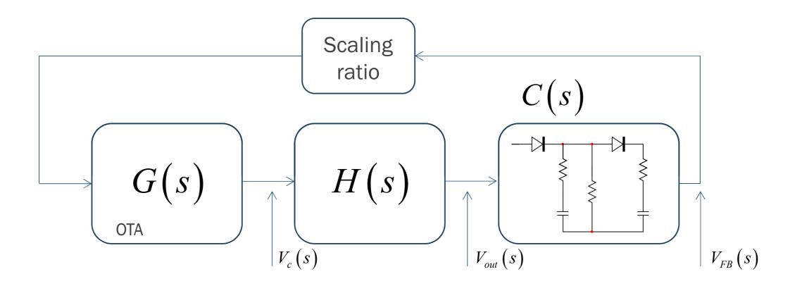
The second transfer function C(s) is cascaded with that of the plant to form the dynamic response we need. From this response and based on the requirement (crossover frequency and phase margin), we can deduce a compensation strategy.
