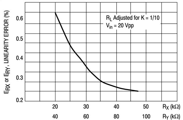
Figure 14. Linearity versus  $R_X$  or  $R_Y$  with  $K = 1/10$
