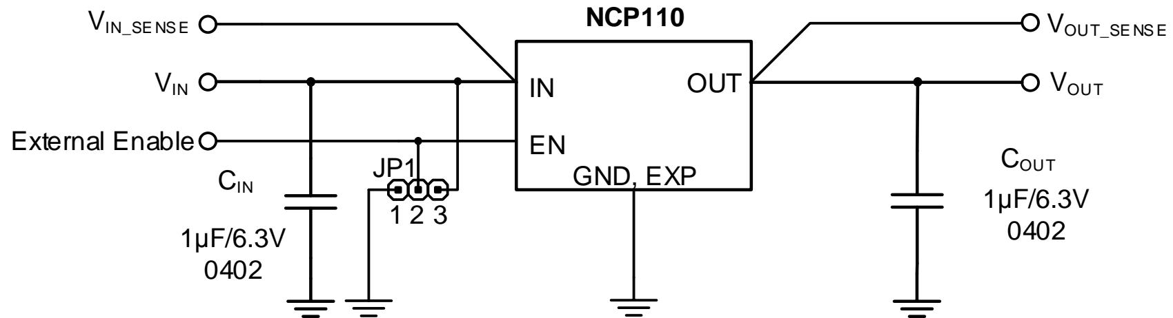
The NCP110 is 200mA low  $V_{IN}$ , low noise, high performance LDO with low quiescent current (25 $\mu A$  max.) and very high PSRR. The NCP110 also offers excellent load/line transients and ultra-low noise.
