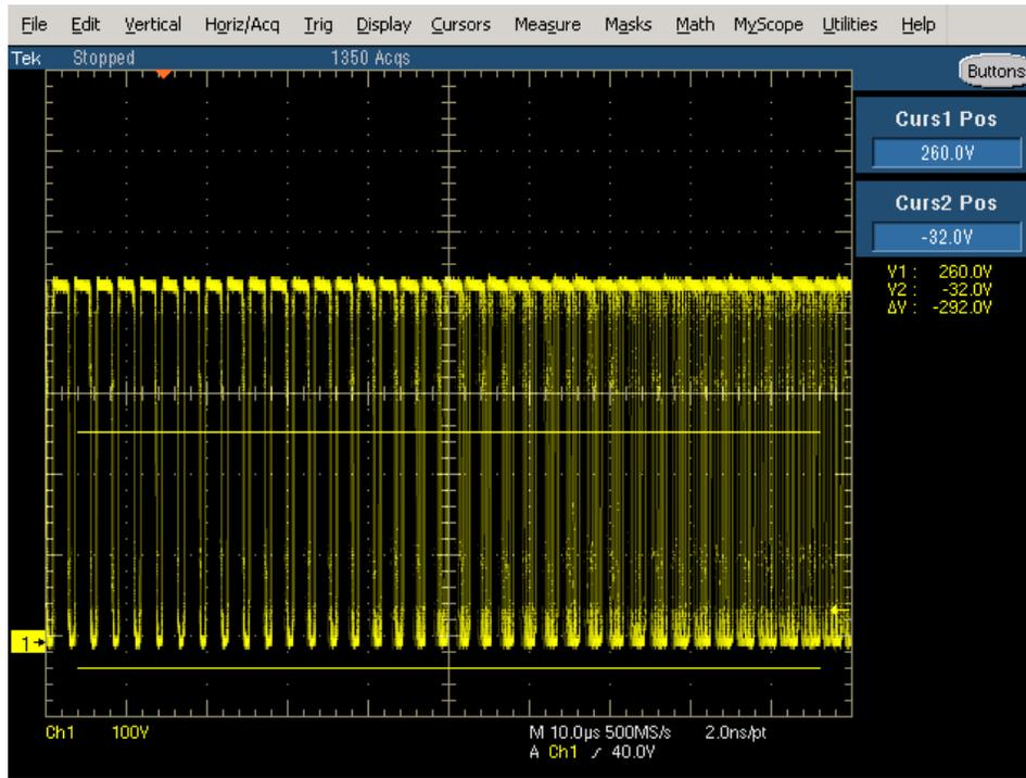
Figure 3 - Clean CCM Operation
