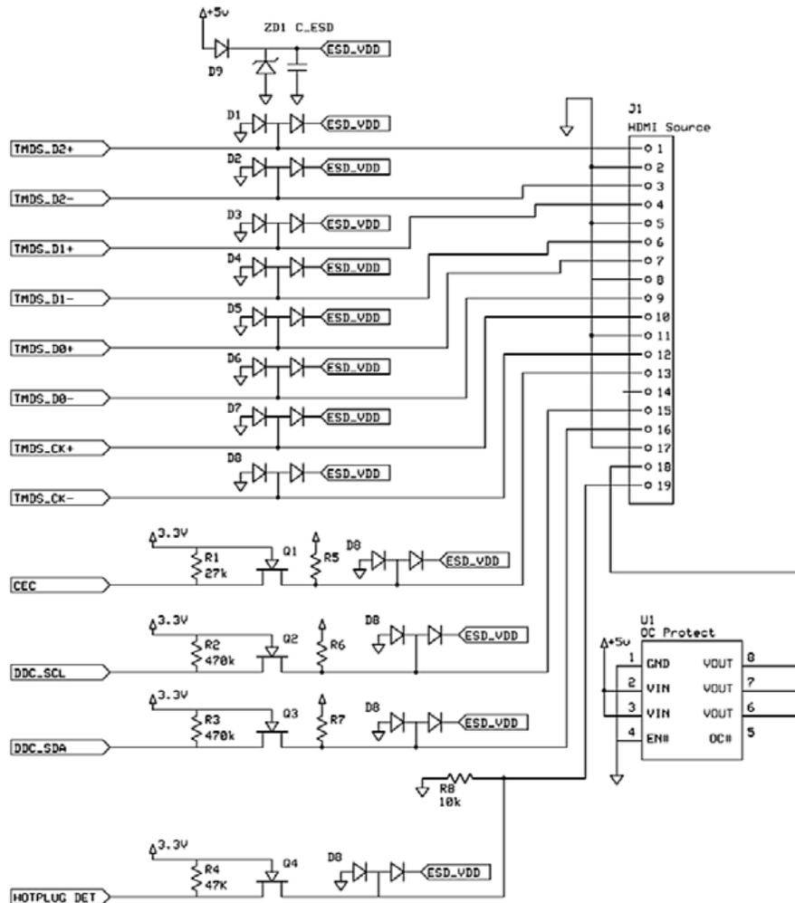
Here, each TMDS line is protected from ESD with a low-capacitance Dual Rail Clamp diode pair that routes negative ESD pulses directly into ground, and positive pulses back to ground through a zener diode. Each of the signal lines exposed to the HDMI connector are protected in this manner. All of these clamps are further prevented from providing a DC backdrive path through a blocking circuit from the biasing supply.
