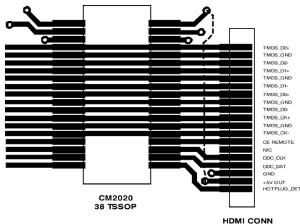
The sample layout shown above demonstrates the ultra-compact nature of the solution in relation to the size of a typical SMT HDMI connector (CM2020 Source side shown here.) The 0.5 mm pitch of the TSSOP-38 package lines up directly with the connector, and provides 10 short ground return paths from TMDS diode clamps to minimize total inductance. This close proximity to the connector also maximizes ESD protection by shunting the harmful pulses before they travel through the PCB.
