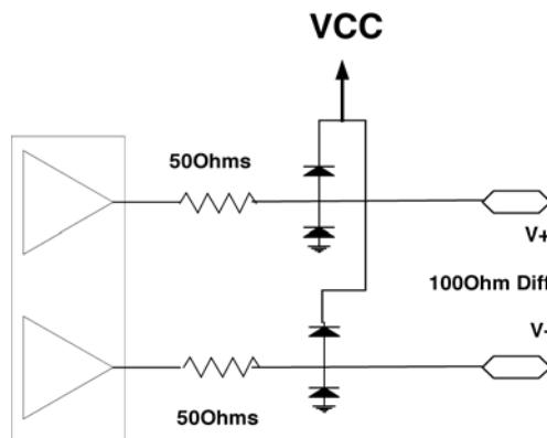
The channel capacitance of the reverse biased ESD clamp diodes and the parasitic series inductance of the package leads and bond wires (shown below) create a lumped resonant LC tank circuit that creates a low impedance shunt at the natural self-resonance frequency of the device.
