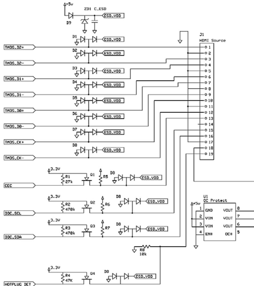
Here, each TMDS line is protected from ESD with a low-capacitance Dual Rail Clamp diode pair that routes negative ESD pulses directly into ground, and positive pulses back to ground through a zener diode. Each of the signal lines exposed to the HDMI connector are protected in this manner. All of these clamps are further prevented from providing a DC backdrive path through a blocking circuit from the biasing supply.
