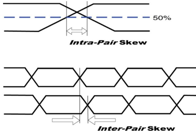
The HDMI Specification, Version 1.1 specifies "Intra-Pair Skew at Source Connector," at a maximum of  $0.15 \times T_{bit}$ , or less than about 90 ps @ 1.65 GHz. "Inter-Pair Skew at Source Connector" is a more "relaxed"  $0.20 \times T_{pixel}$ , or less than about 1.2 ns @ 165 MHz.
