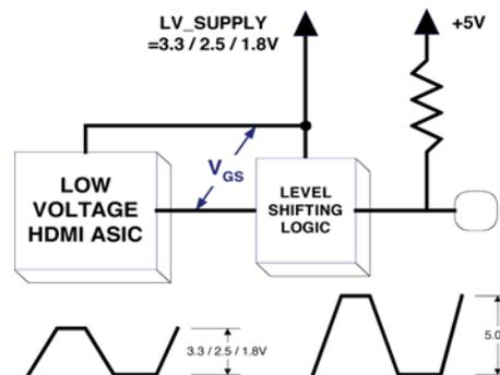
Simple NFET level translation techniques use the bidirectional nature of the FET and the low threshold voltage to "clamp" the lowside of the protection block to a reference voltage, such as the VDD of the low-voltage ASIC. Unexpected glitches and peaks that might normally destroy these integrated "tolerant" structures are easily absorbed by the relatively higher power external devices.
