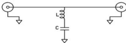
The impedance at this resonant frequency and the quality factor (Q) of the insertion loss notch determine how much this resonance point will distort the signal. The following plot shows the range of possible resonant frequencies for a SOT-23-6 package with 1.0 to 1.5 pF of channel capacitance (approximately 3.1 GHz with 1.5 pF to 4.2 GHz with 1.0 pF).
