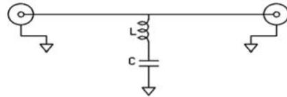
The impedance at this resonant frequency and the quality factor (Q) of the insertion loss notch determine how much this resonance point will distort the signal. The following plot shows the range of possible resonant frequencies for a SOT-23-6 package with 1.0 to 1.5 pF of channel capacitance (approximately 3.1 GHz with 1.5 pF to 4.2 GHz with 1.0 pF).
