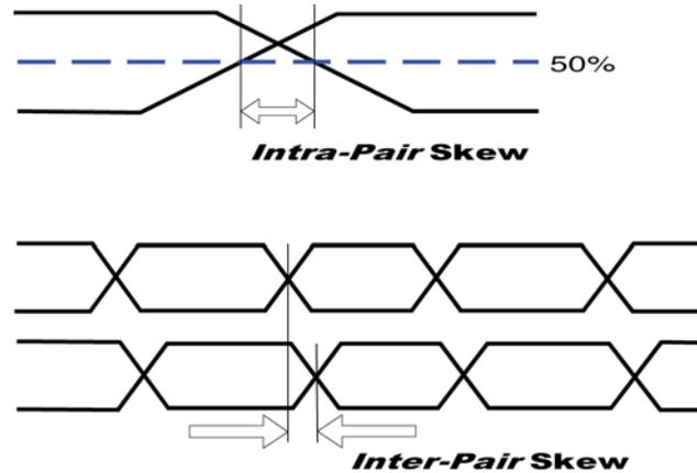
The HDMI Specification, Version 1.1 specifies "Intra-Pair Skew at Source Connector," at a maximum of  $0.15 \cdot T_{bit}$ , or less than about 90 ps @ 1.65 GHz. "Inter-Pair Skew at Source Connector" is a more "relaxed"  $0.20 \cdot T_{pixel}$ , or less than about 1.2 ns @ 165 MHz.
