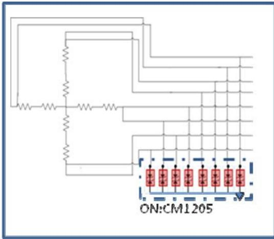
Figure 8. 8-wired Touch Screen with External ESD Protection
