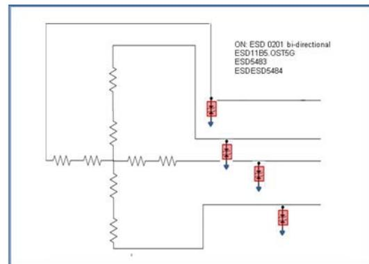
Figure 7. 4-wired Touch Screen with External ESD Protection
