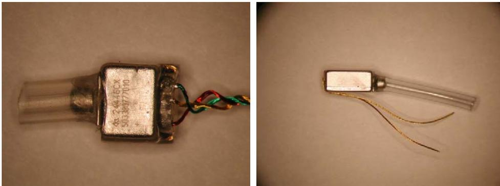
It will be necessary to trim the acoustic tubing for the receiver as shown below.
