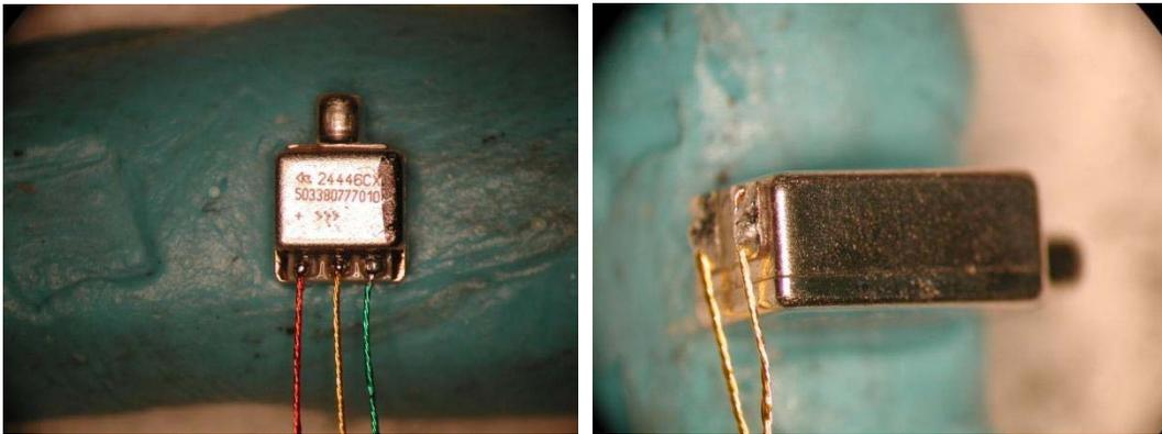
The transducers should be pre wired and sealed with heat shrink as shown in the figures below:
