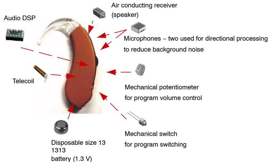
**Figure 2. BTE Hearing Aid Components**
