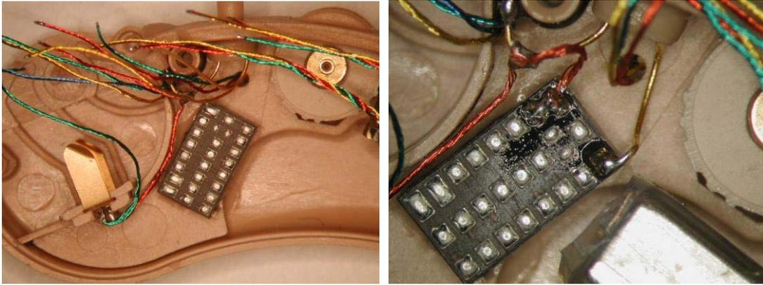
Components should be stabilized with a non-adhesive putty to allow easy access for soldering to the component pins.
