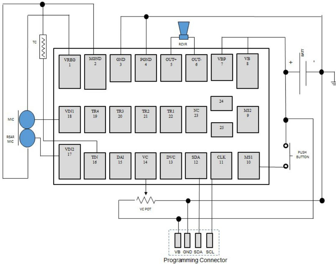
**Figure 4. BTE Schematic Diagram**
