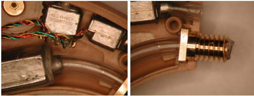
The telecoil is directly attached to the SB3231 TIN inputs using short wires to minimize noise coupling into the analog microphone inputs.
