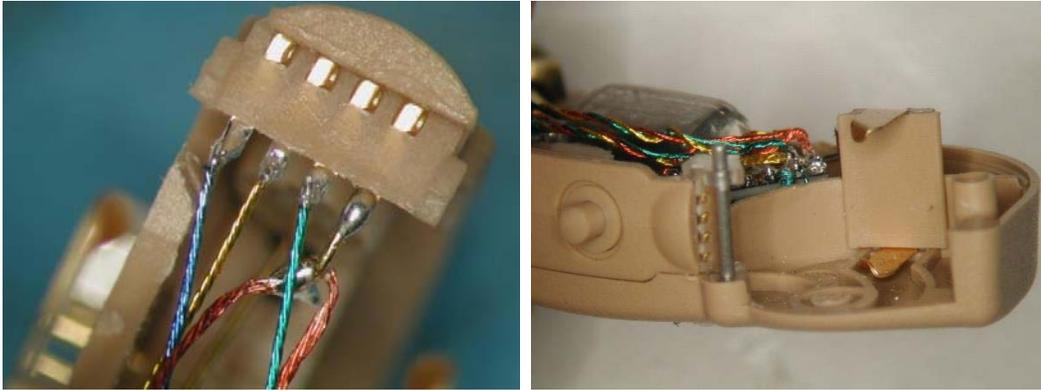
Star routing of the power supply lines back to the battery is performed to minimize noise and crosstalk in the system.
