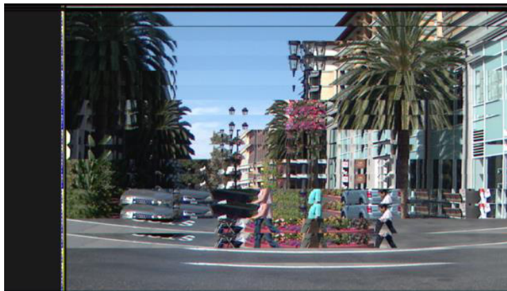
Figure 6. Example of a Fault in the Row Addressing Logic
