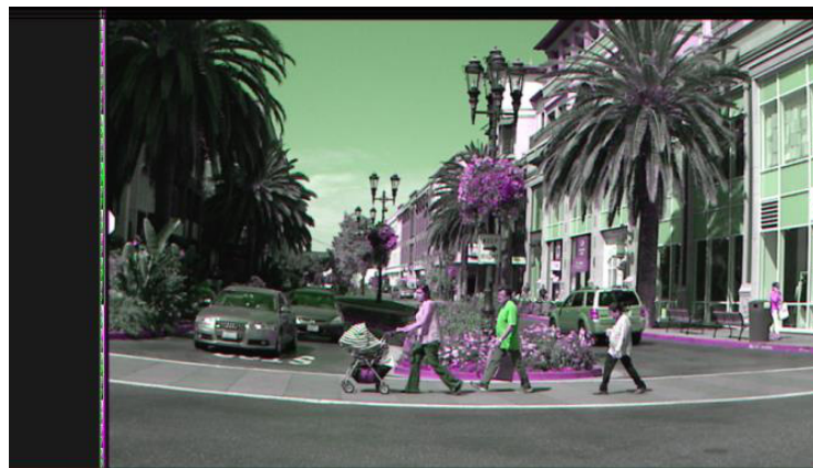
Figure 5. Example of a Color Error due to an Image Pipeline Fault
