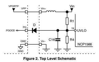
Recommended part numbers for this diode (reference designator D in Figure 2) are BAS70L, NSR02100 or eventually BAS70SL.
