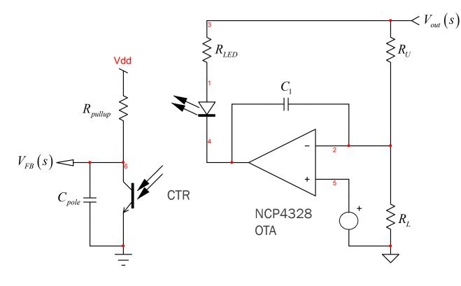
For this type 2 compensator (1 pole at the origin, 1 zero and 1 pole), a single capacitor  $C_1$  is necessary. The second capacitor  $C_{pole}$ creates the needed pole for rolling off the gain at high frequencies.
