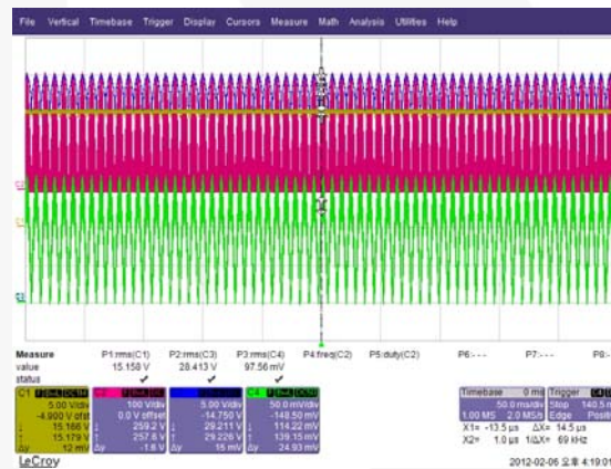
CH1: V CC , CH2: V DRAIN , CH3: V LED , CH4: I LED
