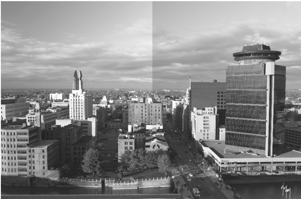
Figure 1. Dual Output CCD (Left/Right) Image with No Seam Correction
