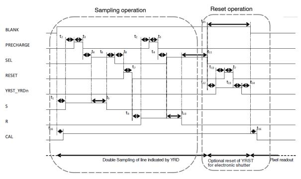
Note that the "Sampling operation" indicated above resets the photodiode after the S-value has been sampled, so that and R value may be provided for uncorrelated double sampling. Hence, each line operation contains two resets: One for the photodiode being read out, and a second for the photodiode on the reset-line.
