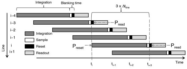
Figure 4. Rolling Shutter Operations Illustrated in Line-per-line Form
