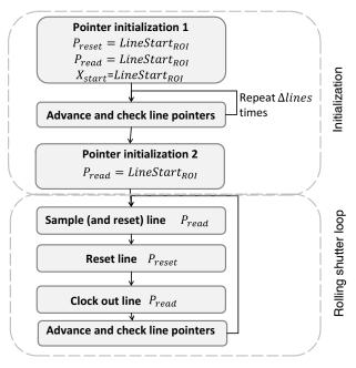
Note that two lines are reset during a step of the rolling shutter loop: First the P.read line is reset to provide the R-value for the readout. Secondly, the line P.reset is reset in order to control the integration time.
