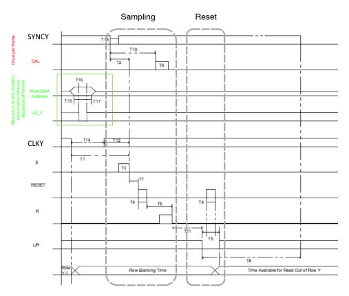
Note that the "Sampling operation" indicated above resets the photodiode after the S-value has been sampled, so that and R value may be provided for uncorrelated double sampling. Hence, each line operation contains two resets: One for the photodiode being read out, and a second for the photodiode on the reset-row.
