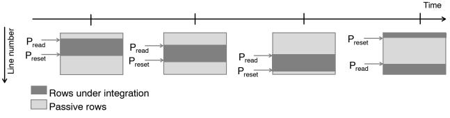
Figure 5. Illustration of Rolling Shutter Principle
