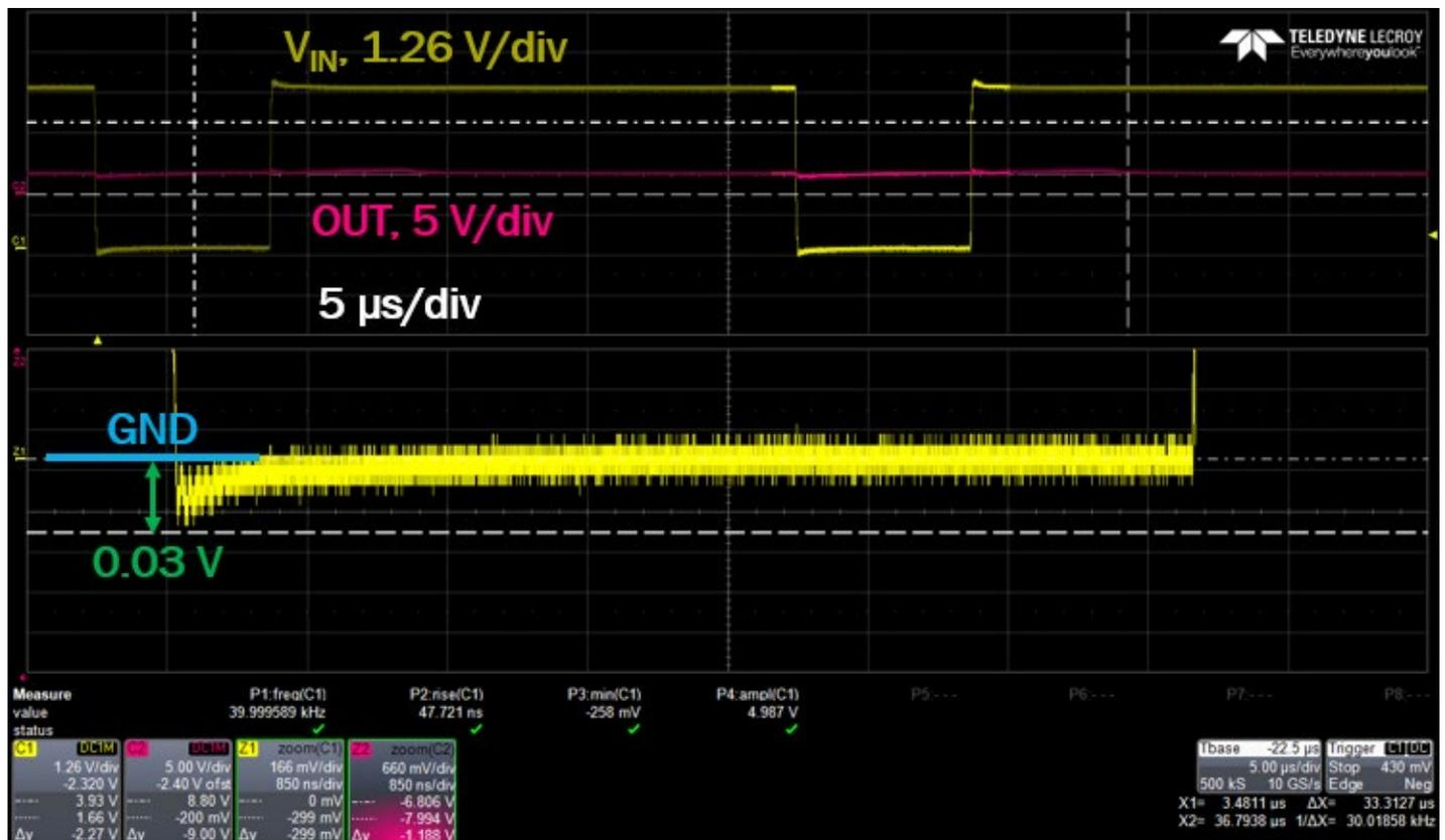
Figure 6: Zoom view of Figure 5. Overshoot reduced to -0.3 V, which is right at the lower side of the ABS Max spec limit.
