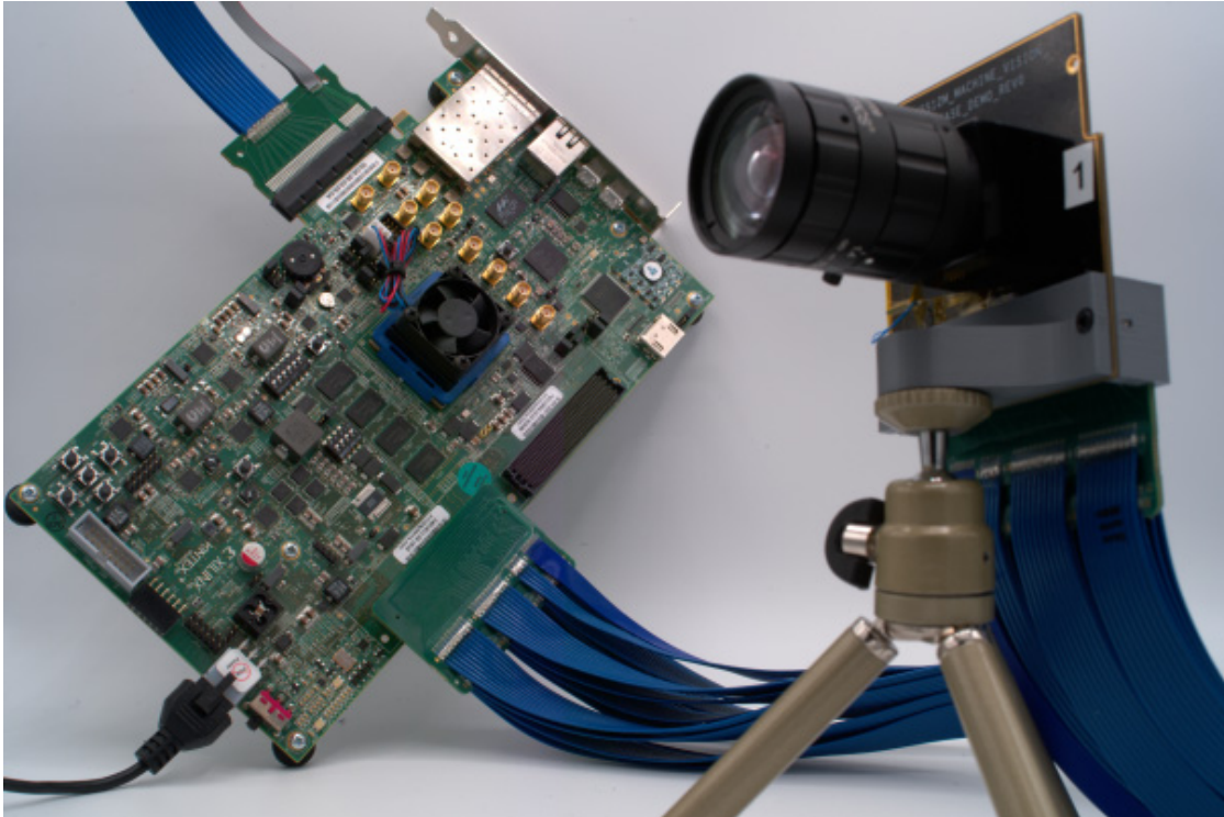
Figure 9. X-Celerator Development Kit (lens not included) Connected to a Xilinx KCU105 Development Platform (not included)
