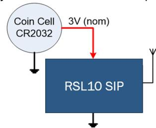
Figure 1: RSL10 System in Package (RSL10 SIP) without a sensor companion
