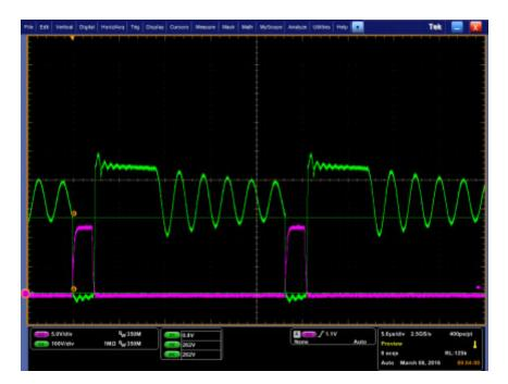
Figure 7. Valley Switching at 6<sup>th</sup> Valley for Improved Efficiency (Green: Drain voltage, Purple: Drive)
