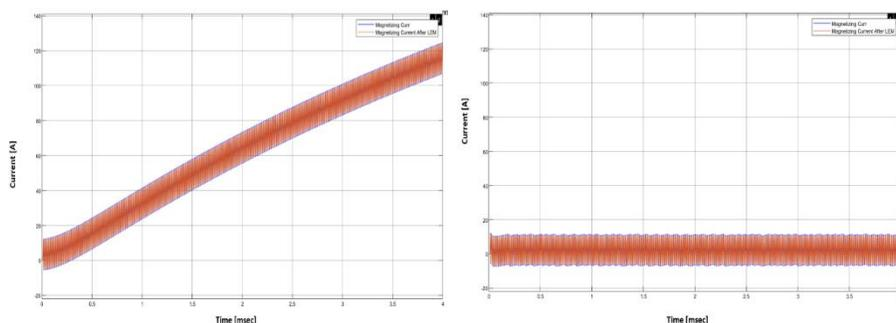
Fig. 17. Simulated transformer magnetizing current ( $I_M$ ) with the flux-compensation algorithm inactive (left) and active (right) of the DAB. When no flux-balancing technique is running, the residual dc current is building up during each switching cycle, which will eventually saturate the core.
