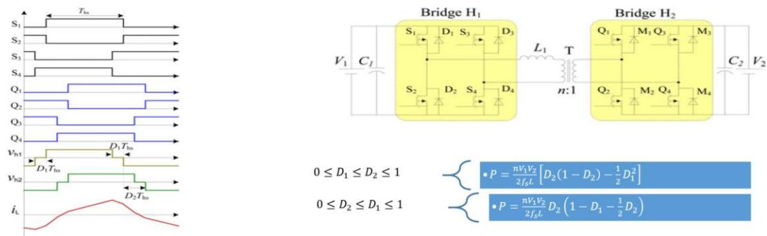
Fig. 13. Dual phase-shift (DPS) technique. (Source: "Overview of Dual-Active-Bridge Isolated Bidirectional DC-DC Converter for High-Frequency-Link Power-Conversion System"<sup>[9]</sup>)
