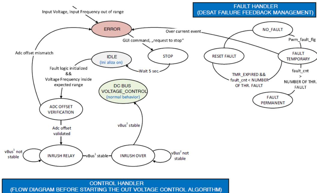
Fig. 7. Overview of the state machine for the PFC converter.
