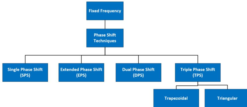
Fig. 11. Classification of different phase-shift techniques. Triple phase-shift (TPS) is a unified version of the other techniques, and each of these can be considered as a subcase of TPS.
