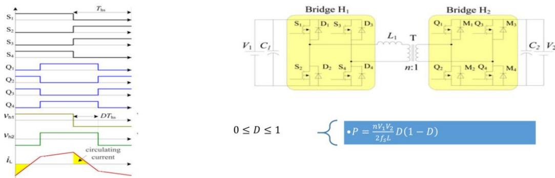
Fig. 12. Single phase-shift (SPS) technique. (Source: "Overview of Dual-Active-Bridge Isolated Bidirectional DC-DC Converter for High-Frequency-Link Power-Conversion System"<sup>[9]</sup>)
