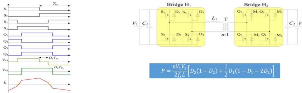
Fig. 14. Extended phase-shift (EPS) technique. (Source: "Overview of Dual-Active-Bridge Isolated Bidirectional DC-DC Converter for High-Frequency-Link Power-Conversion System"<sup>[9]</sup>)
