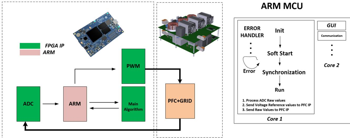
Fig. 2. Overview of the 25-kW PFC converter control architecture. Tasks are distributed between the FPGA and ARM MCUs in the Xilinx Zynq 7000 on the UCB. The control architecture overview will be similar for the DAB converter.
