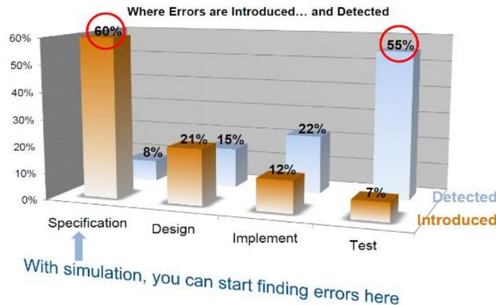
Fig. 3. Errors introduced versus errors detected. (Source: Clive Maxfield and Kuhoo Goyal’s book, “EDA: Where Electronics Begins.”)
