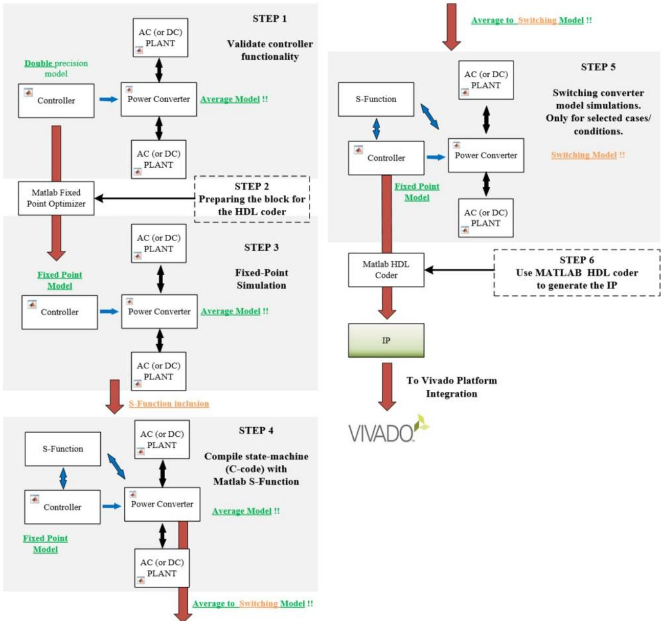
Fig. 6. Flow chart of the six steps in the simulation model development stage. For ease of representation, the "peripherals" block in Fig. 5 has been omitted from this flow chart. It would be present in the same position and connections with the other blocks as in Fig. 5.
