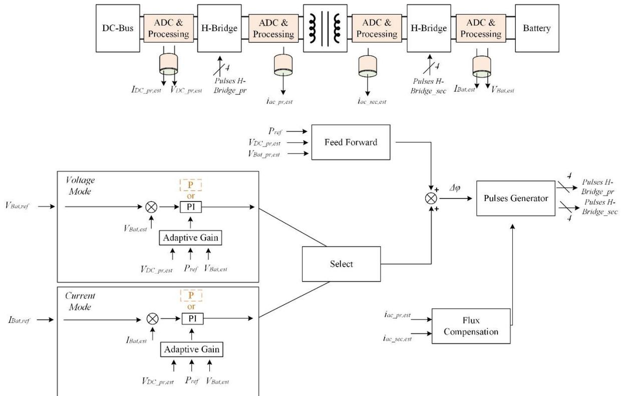
Fig. 15. Block diagram of the DAB control algorithm. The transformer flux-balancing algorithm is included in it as well.
