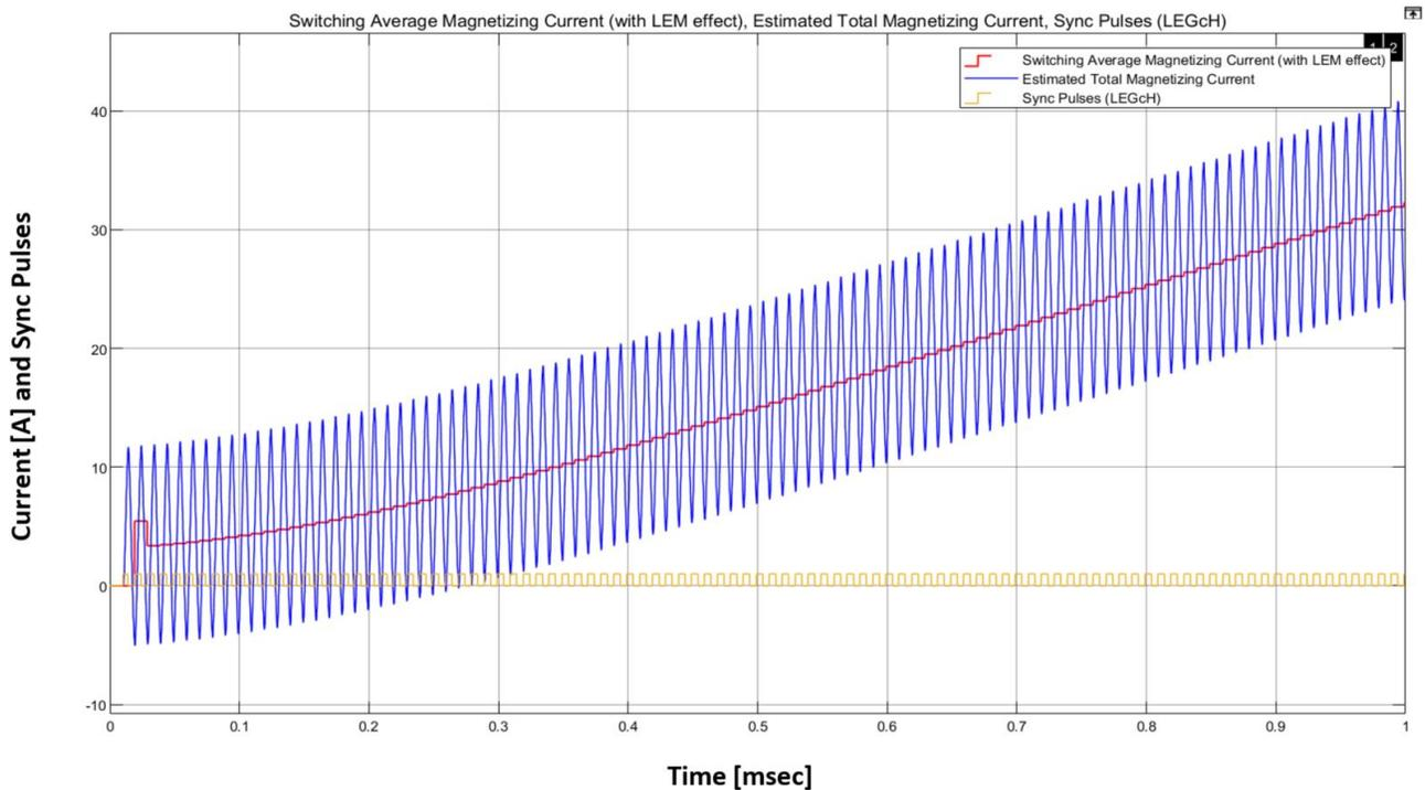
Fig. 20. Estimated total magnetizing current (with LEM current sensor effect), estimated switching average (with LEM sensor effect), and synchronization pulses. Flux-balancing algorithm is inactive in this simulation.
