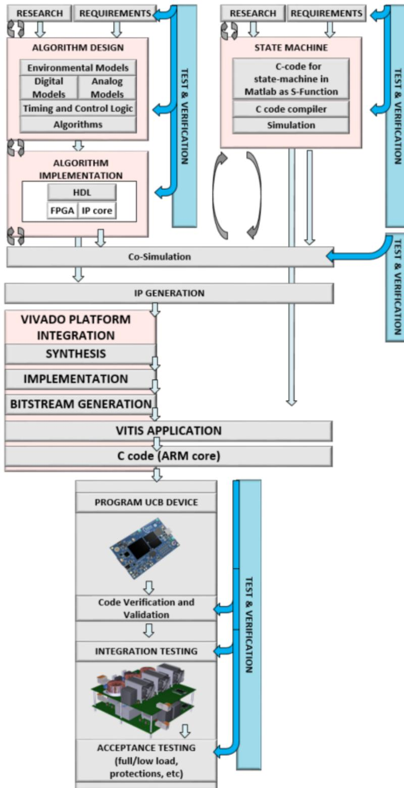
Fig. 4. Firmware development flowchart for the 25-kW fast dc EV charger.
