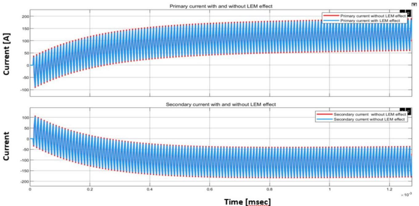
Fig. 18. Primary and secondary current measurement with and without the LEM current sensor effect. The flux-balancing algorithm was not active in this simulation.
