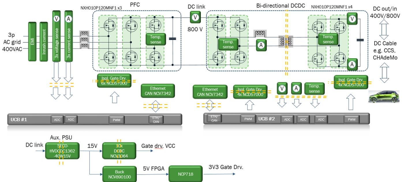
Fig. 1. A high-level block diagram of the 25-kW EV dc charger.
