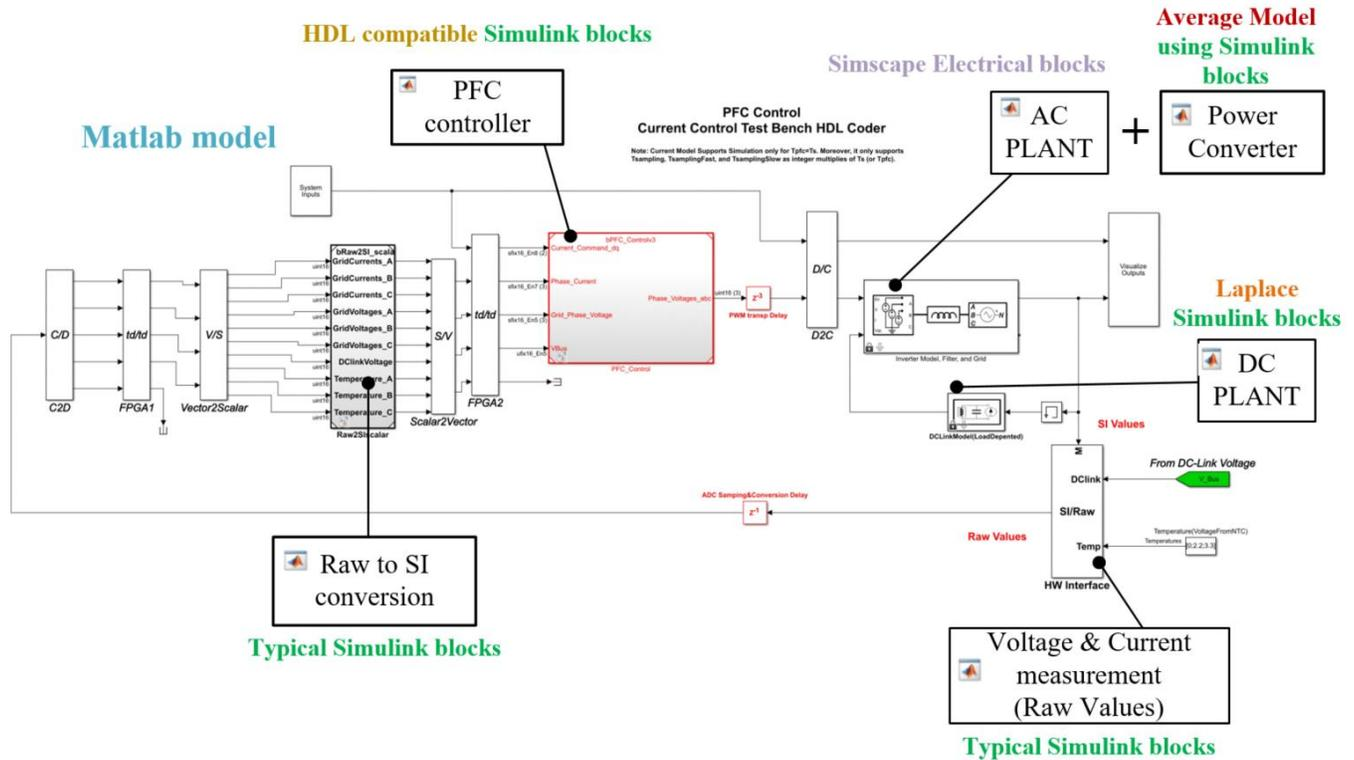
Fig. 10. Main PFC controller Simulink model. The dc plant block (simple resistor and capacitor) is used as a load to test the PFC algorithmic functionality, and does not represent a model for the actual DAB converter.
