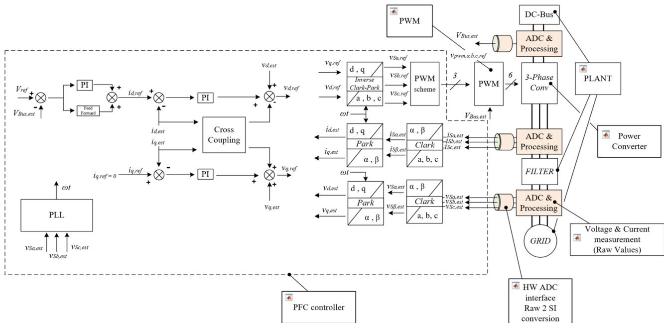
Fig. 9. Detailed block diagram of the PFC control algorithm.
