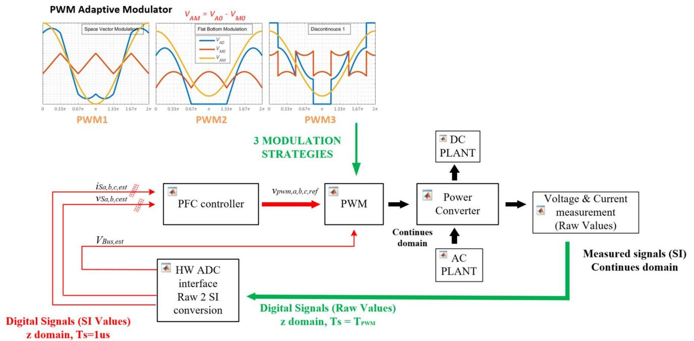
Fig. 8. High-level block diagram of the PFC control algorithm.
