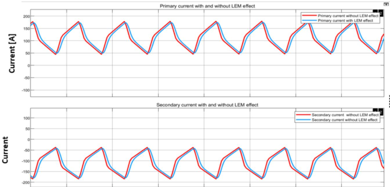
Fig. 19. Primary and secondary current measurement with and without the LEM current sensor effect.
