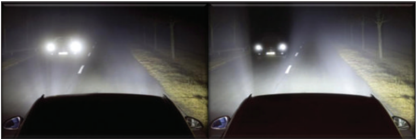
Figure 2: Comparison of AFS Implementations (left) with anti-glare high beams using Pixel Light and without (right).
